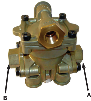
PPV CLOSING PRESSURE 70 PSI CRACK PRESSURE 4 PSI
